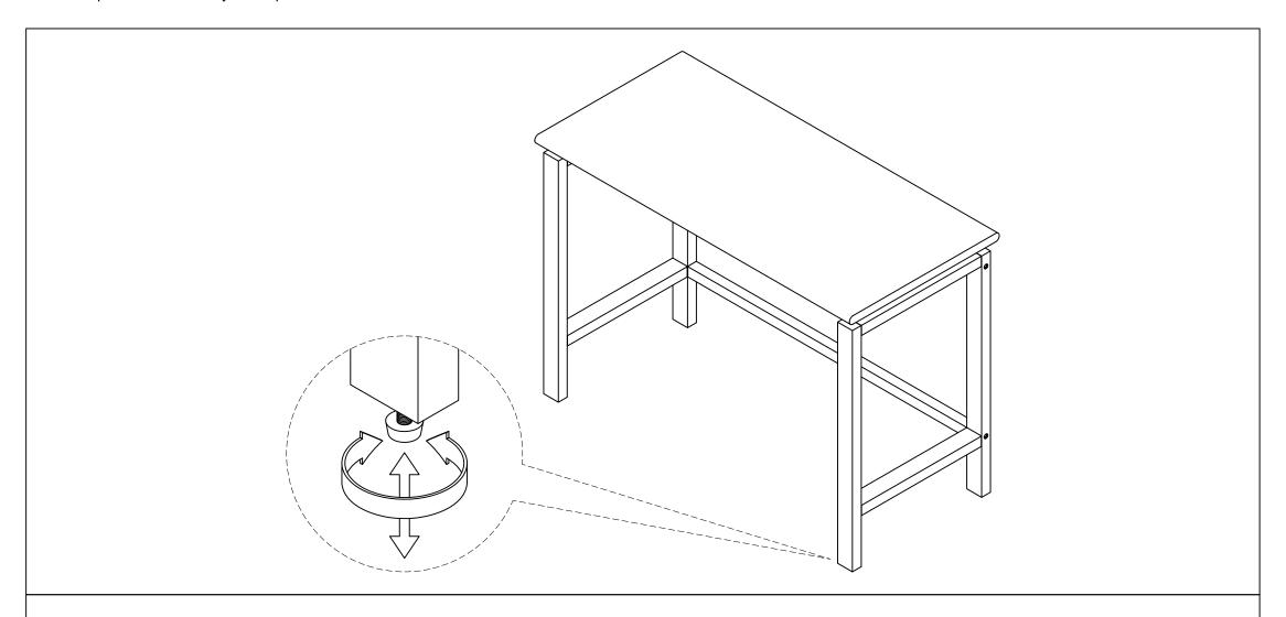
STEP 9 ADJUST THE ADJUSTER BOLT THAT HAS ALREADY ASSEMBLED TO THE LEGS TO STABILIZE YOUR UNIT.
