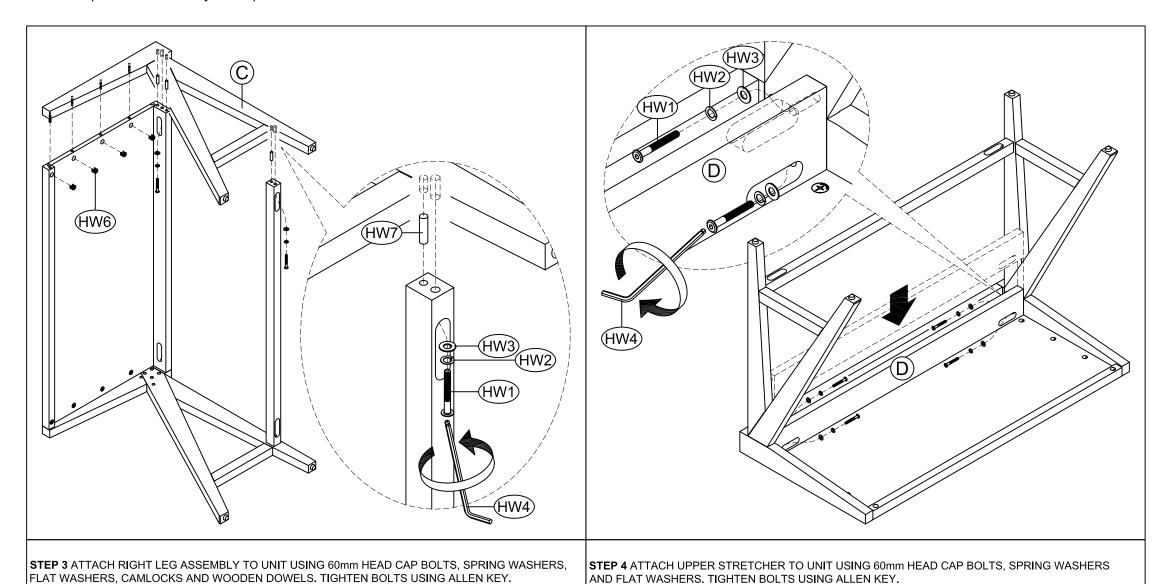
AND FLAT WASHERS. TIGHTEN BOLTS USING ALLEN KEY.
