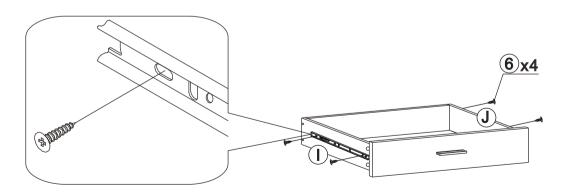
**STEP11:** Attach small part of part (M) to (I), (J) using HW(6).
