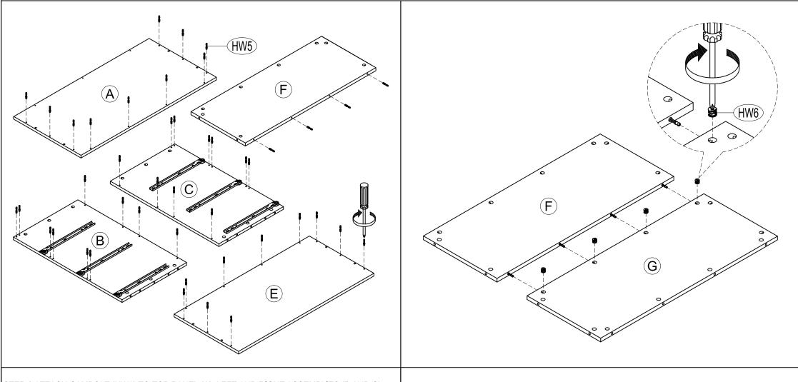
STEP 1 ATTACH CAMBOLT (HW5) TO TOP PANEL (A), LEFT AND RIGHT ASSEMBLIES (B AND C), BOTTOM PANEL (E) AND UPPER BACK PANEL (F).
