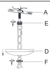
**Step 4:** Seperate the Mounting Plate(A) from the Canopy(D) by turning the Canopy Nut(F) anti-clockwise.
