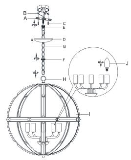
**Step 5**: Install the Mounting Plate(A) to the junction box with Mounting Screw (C), Attach the Canopy(D) to the junction box and fix it by turning the Canopy Nut(F) clockwise, Insert the bulbs (J) into the Sockets
