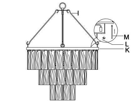
**Step 6**: Insert the light bulb (L) into the lamp Sockets. Insert the clear glass (M) on the lamp body (K).
