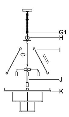
**Step 2**:Put ring (H) was twisted into the light frame (J) and then the iron hook (I) was attached to the ring (H), lamp body (K). Put the closable link(G1) onto the fixture loop(H).
