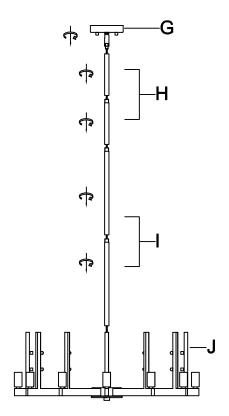
**Step 2**:Screw the long stem(I) and Short Stem (H) to the Lamp Body (J). Make sure to feed the branchwires of the fixture through the stems during assembly. Remove or add stems to adjust the height. Then screw the canopy (G) to the stem.
