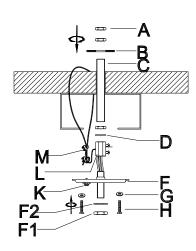
**Step 1:** Raise the threaded rod (C) thread to the cluster (L), then attach to the ceiling, secure with metal washer (B) and hex nut (A). Wrap the steel wire rope around the beam and lock it with the steel cable buckle. Attach the mounting bracket (F) to the cluster (L), then install the mounting bracket (F) to the junction box with plain washer (G) and outlet box screw (H), finally secure the mounting bracket (F) with teeth washer (F2), hex nut (F1).
