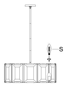
Step 6: Install the light bulb (S) to the socket.
