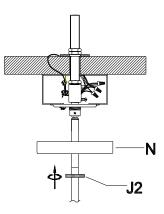
Step 4: Attach the canopy (N) to the ceiling with canopy ring (J2).
