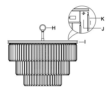
**Step 6**:Insert the light bulb (J) into the lamp Sockets. Insert the crystal bar (K) on the lamp body (I).
