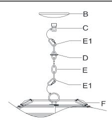
Step 1:Connect the metal chain (E) by locking the collar loop (C) with the lock link (E1) on the top and lock the fixture body (F) with the lock link (E1) on the bottom.
