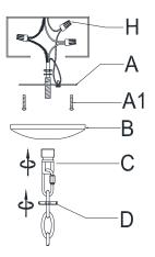
Step 3: Attach the mounting bar(A) to the junction box with outlet box screw (A1). Attach the canopy (B) to the mounting bar (A), secure with the collar loop (C) and canopy ring(D).
