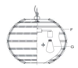
Step 4: Install the light bulb (G) to the socket.
