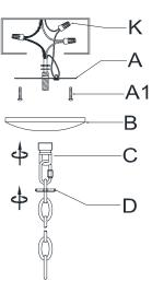
**Step 4:** Attach the mounting bar(A) to the junction box with outlet box screw (A1). Attach the canopy (B) to the mounting bar (A), secure with the collar loop (C) and canopy ring(D).
