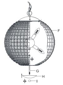
**Step 6:** Raise the threaded rod (G) thread to the fixture body, attach the metal cup (H) to the bottom of fixture body, finally secure with ball nut (I).
