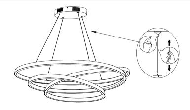
**Step 4:** Press the expansion piece and adjust the height of the lamp body. Turn on the light and adjust the brightness.
