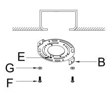
**Step 1:**Fix the mounting bracket(B) to the outlet box with mounting screw(F).
