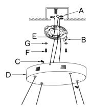
**Step 3:** Carefully remove packaging from fixture, adjust wire length to desired mounting height, fix the canopy(D) to bracket(B) using maching screw(C).
