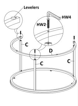
\*Do not fully tighten the bolts until the product is assembled.
