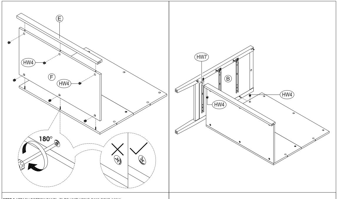
STEP 3 ATTACH BOTTOM PANEL (F) TO UNIT USING CAMLOCKS (HW4).
