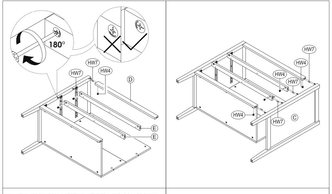
STEP 5 ATTACH TOP FRAME (D) AND BOTTOM FRAMES (E) TO UNIT USING CAMLOCKS (HW4) AND DOWELS (HW7).
