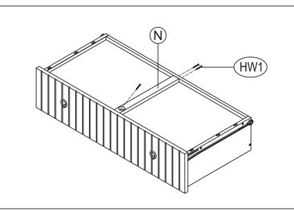
STEP 10 ATTACH DRAWER SUPPORTS (N) TO THE BOTTOM SIDE OF DRAWERS
