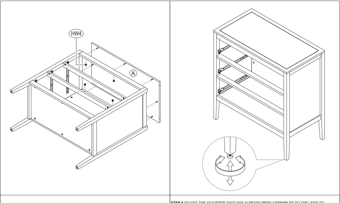
STEP 7 ATTACH TOP PANEL (A) TO UNIT USING CAMLOCKS (HW4).
