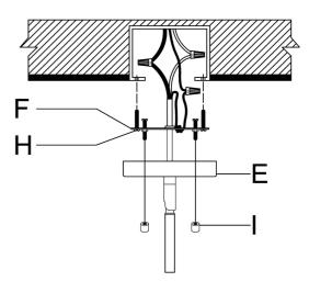
**Step 4:** Fix the Mounting Plate(F) to the junction box with Mounting Screw (H).
