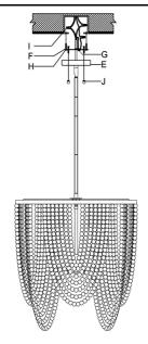
**Step 5:** Attach the Canopy(E) to the junction box and fix it by turning the Canopy Nut(J) clockwise.
