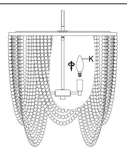
**Step 6:** Insert the bulbs (K) into the Sockets.
