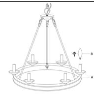
Step 6: Insert the Bulbs (B) into the socket.
