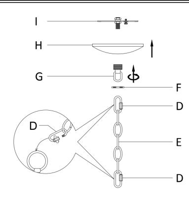
**Step 1:** Unpack all parts from cartons carefully. Place the Canopy(H)onto the Hanging Loop(G), Place the tube of Mounting Plate(I)into the theaded portion of the Hanging Loop(G) and fix it by turing the Canopy, Nut(F) clockwise till tight. Attach the Closable Link(D) onto the Hanging Loop(G)
