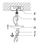
**Step 5:** Tuck wires inside junction box. Attach the Canopy (H) to the junction box and fix it by turning the Canopy Nut (F) clockwise.
