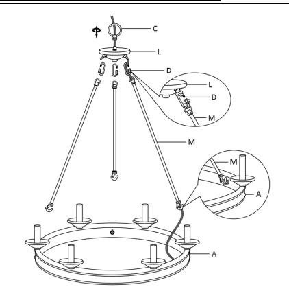
**Step 2:** Thread Fixture Loop (C) to Loop Assembly (L). Respectively attach the Closable Link(D) onto the loop of the Loop Assembly (L) and Connecting Rod (M), then respectively attach clip of the Loop Assembly (L) to ring of the Lamp Body (A).
