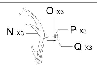
**Step 1:** Unpack all parts from cartons carefully. Unscrew the Hex Nut (Q), Spring Washer (P) and Washer (O) from the Branch (N).
