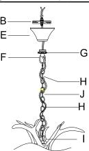
**Step 4:**Weave the 2 wire power cord and bare ground wire through every other loop to the top of chain(J),center holes of Hanging Loop(F)&Canopy(E)&Mounting Plate(B) as diagram.
