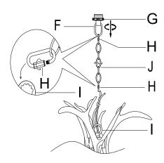
**Step 3:** Screw the Chain(J) to the Hanging Loop(F) and the Fixture Loop (I) with Closable link/cap (H) as diagram.
