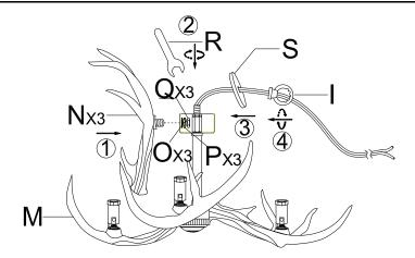
**Step 2:** Insert the threaded portion of the Branch (N) into the topper hole of the Lamp Body (M), attach Washer (O), Spring Washer (P) and fix it with Hex Nut (Q), rotating the Hex Nut (Q) clockwise by Wrench (R) till tight. Place the Cover (S) and fix it by turning the Fixture Loop (I) clockwise till tight.
