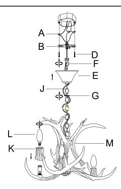
Step 6: Attach the Mounting Plate (B) onto the junction box by inserting two Mounting Screws (D) and turning clockwise till tight. Slide the Canopy (E) upward along the chain(J) till the ceiling surface. Fix the Canopy(E) by rotating the Canopy Nut(G)clockwise to engage it with the threaded portion of the Hanging Loop (F) until secure. Do not over tighten this nut. Place each Socket Sleeve(K) onto each socket until secure. Insert the bulbs(L) into the sockets until secure.
