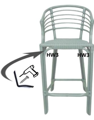
Use piece (hw3) and 8 screw for Top front corner
