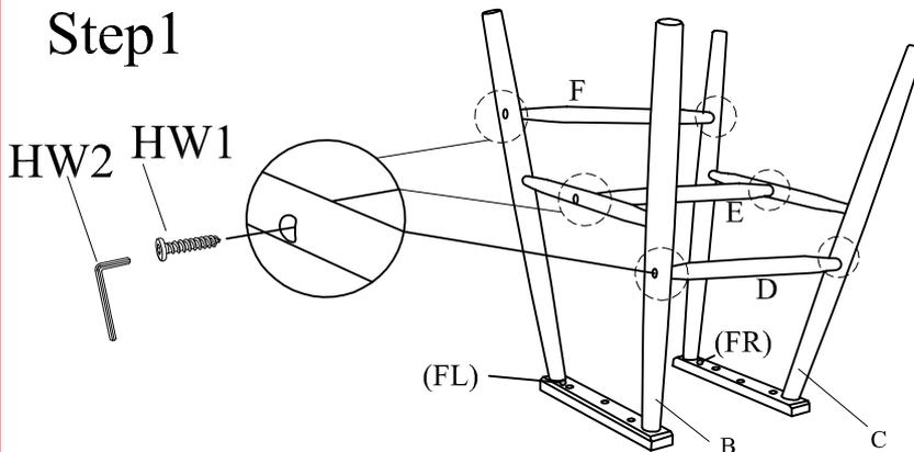
Assemble Short stretcher (D), Middle stretcher (E), and Long stretcher (F) using Screw (HW1) and Allen Wrench(HW2).
