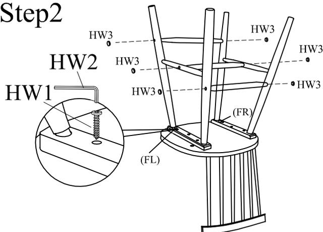
Position the frame assembly into the bottom of chair seat.Align and tighten bolt chair seat and frame using the Screw ( HW1 ) with Allen Wrench ( HW2 ) .
