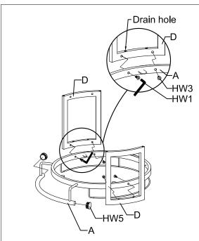
NOTE: Please note there are drain holes in the ring. Please make sure the drain hole faces down in assembly.
