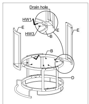
NOTE: Please note there are drain holes in the ring. Please make sure the drain hole faces down in assembly.
