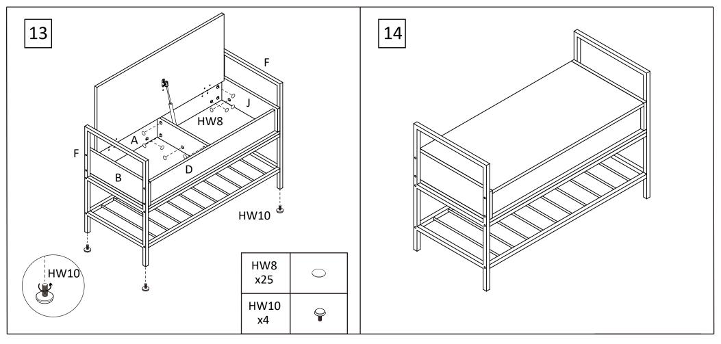
STEP13: Attach 25x stickers (HW8) to panels [A], [B], [D], [J]. Attach 4x adjuster (HW10) to the ends of the legs [F] as shown.
