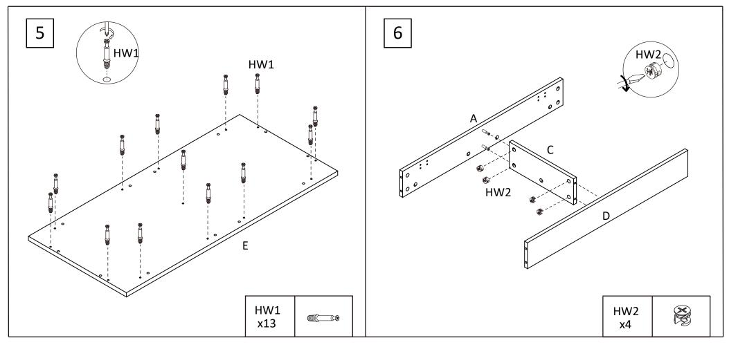
STEP5: Insert 13x cam bolts (HW1) into panel [E]. Tighten with a screwdriver. STEP6: Attach panels [A] and [D] to panel [C] secure with 4x cam lock (HW2). Tighten with a screwdriver.
