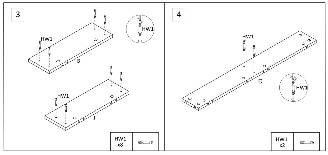
STEP3: Insert 8x cam bolts (HW1) into panels [B] and [J] . Tighten with a screwdriver.
