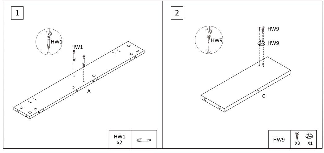
STEP1: Insert 2x cam bolts (HW1) into panel [A]. Tighten with a screwdriver.
