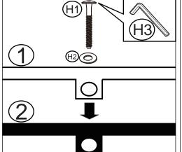
**Step 2 :** Insert bolts in each hole. Tighten them using allen key (provided). Do not over torque bolts.
