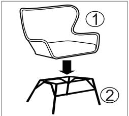
**Step 1 :** Put the seat on top of its base. Follow the arrow head and signs to place it correctly. Align its holes so bolts can be placed properly.
